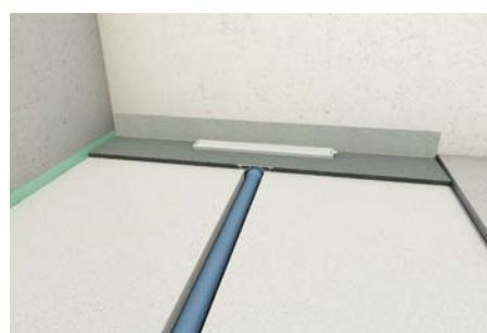
5. Insert the sound insulation and and thermal insulation
