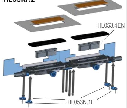
**HL53KV „In|Floor“ vertical drain body for shower channel or short channel**
