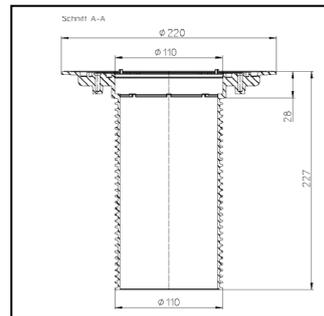
**HL85NH** Extension-element with bitumen flange (drain body)
